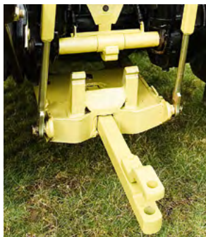
Figure 13: Image of ‘pin and eye’ type coupling. (Image courtesy of Dromone Engineering)
