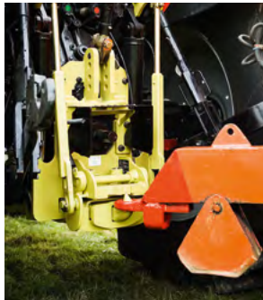
Figure 12: Image of ‘hook and ring’ type coupling. (Image courtesy of Dromone Engineering)
