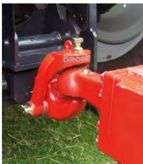
Figure 14: Image of ‘ball and spoon’ type coupling. (Image courtesy of Dromone Engineering)
