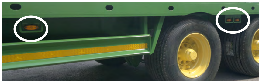
Figure 9: Image of a trailer equipped with modern UN/ECE specification marker lamps. (Image Courtesy of Dooley Bros Engineering Works)
