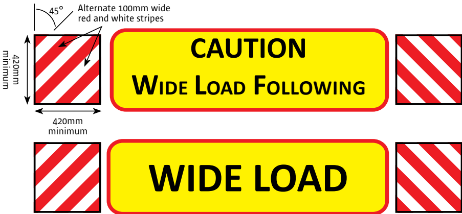
Figure 20: Wide Load Signage to be used when transporting self-propelled equipment over 3.5 metres wide on public roads.
