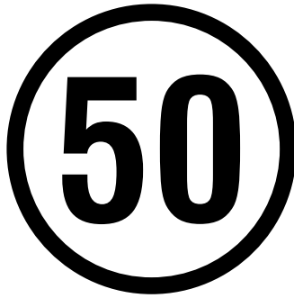
Figure 22: Model speed disc for an agricultural tractor, self-propelled agricultural machine, agricultural trailer or piece of interchangeable towed equipment showing a maximum design speed of 50 km/h.
